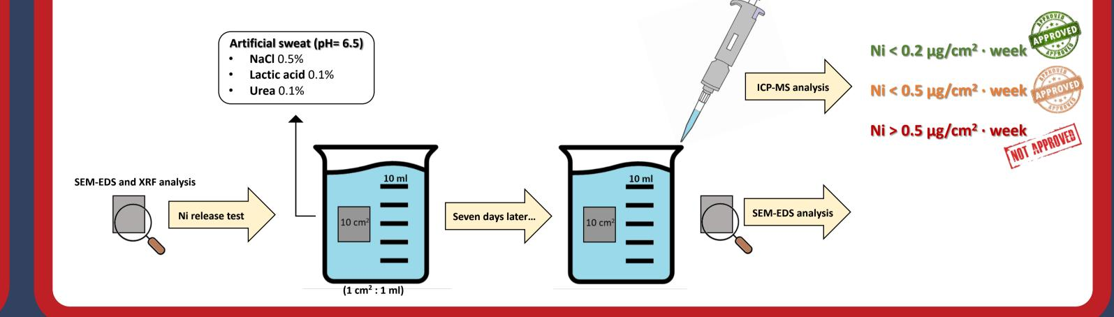
value allowed by current legislation. This is because the steel itself contains nickel (ca. 12% in 316L), so the removal of the surface oxide layer during the electroplating process may facilitate the release of nickel. In this study, we evaluated the nickel release from stainless steel 316L after each galvanization step, starting from surface activation until electroplating processes.
