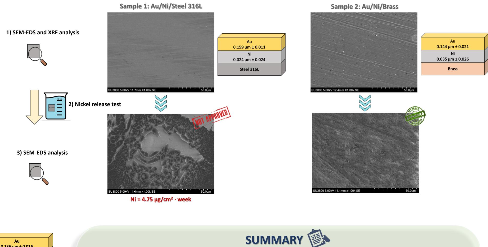
We assessed that stainless steel 316L, as it is, electrochemical degreased and electropolished (surface activation steps), releases nickel below the threshold value allowed by current legislation < 0.2 µg/cm<sup>2</sup> · week.
