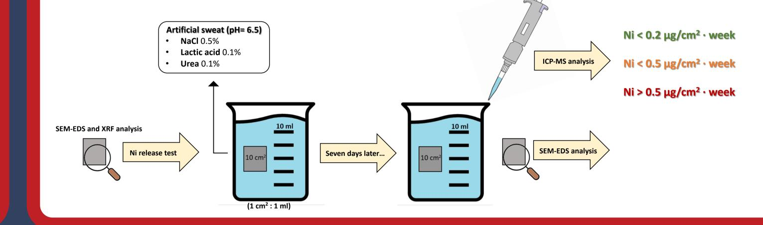
value allowed by current legislation. This is because the steel itself contains nickel (ca. 12% in 316L), so the removal of the surface oxide layer during the electroplating process may facilitate the release of nickel. In this study, we evaluated the nickel release from stainless steel 316L after each galvanization step, starting from surface activation until electroplating processes.
